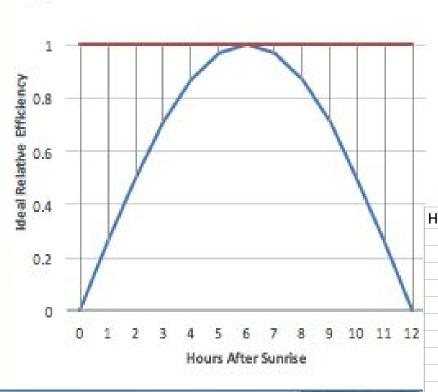
Ideal efficiency chart of Solar Panel Vs. Smart PV by Carl Pennypacker
