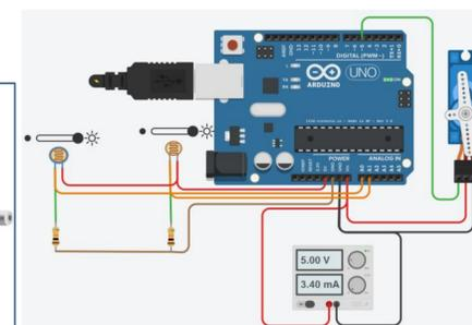
Sample layout of light dependent resistor Arduino wiring.
