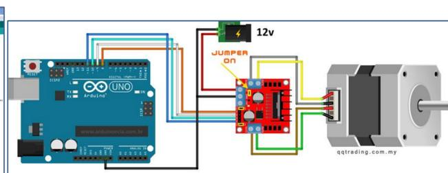
Sample Stepper motor Arduino wiring
