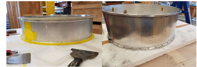
Figure 7: Cryostats before and after application of Aluminum strips
